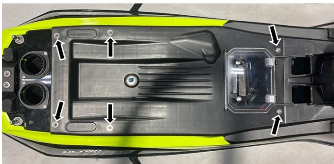
**NOTE: Studs to secure cover in place will be exposed.**
