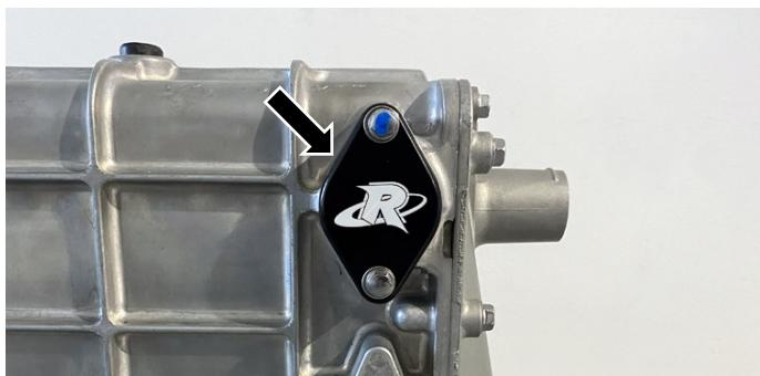
**NOTE: Apply blue Loctite to bolt threads. Torque bolts to 69in•lb (7.8N•m/0.8kgf•m).**
