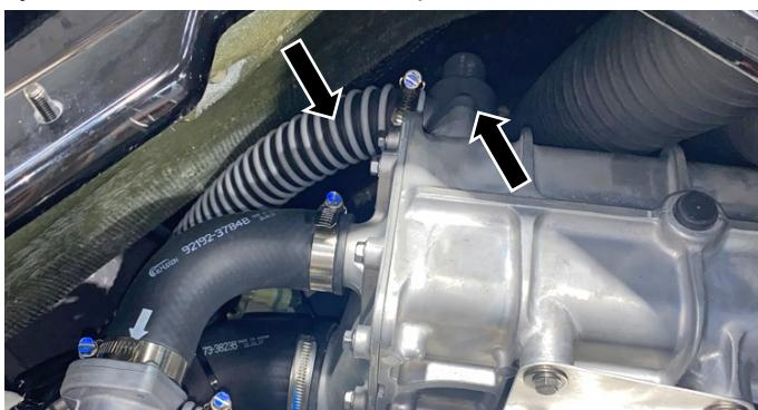
Install supplied vacuum cap onto open fitting on air intake system and secure with supplied zip tie.
